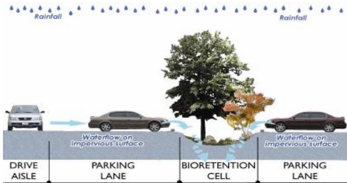
Figure 13.1 Conceptual diagram of a bioretention cell.
