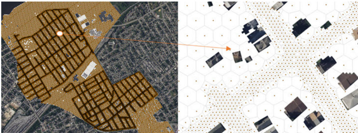
Figure 3 PCSWMM generated 2D mesh of the study area.
